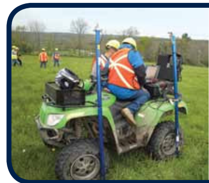
The ATV-mounted mobile control console can also be hand carried and avoids large “doghouses” needed for cabled systems.
